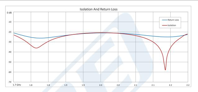
High Power Isolator With 20 dB Isolation From 1.7 GHz to 2.2 GHz, 50 Watts And SMA Female from Pasternack Enterprises has same day shipment for domestic and International orders. Our RF, microwave and millimeter wave products maintain a 99% availability and are part of the broadest selection in the industry.
